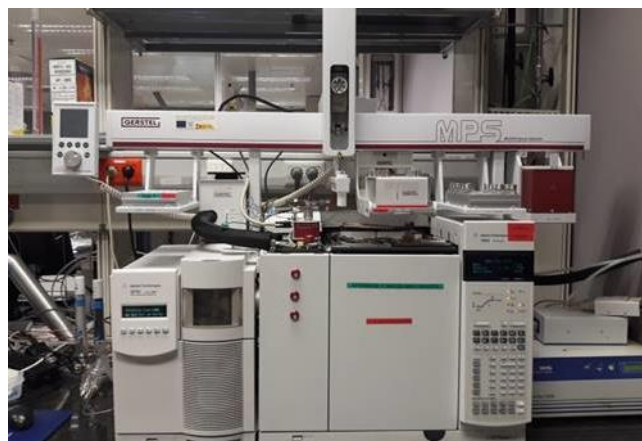
GC-MS with a MultiPurpose Sampler (MPS), Thermal Desorption Unit (TDU) and Pyrolysis Module (PYRO)
